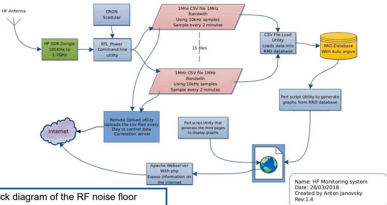
Block diagram of the RF noise floor monitoring system. It can operate on a laptop/PC or a Raspberry Pi
